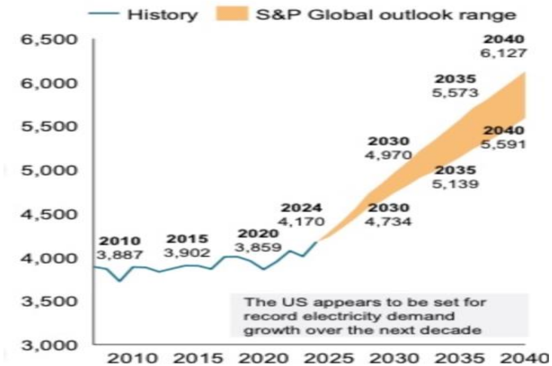
Figure 1.6: US Lower-48 Net On-grid Electricity Demand
