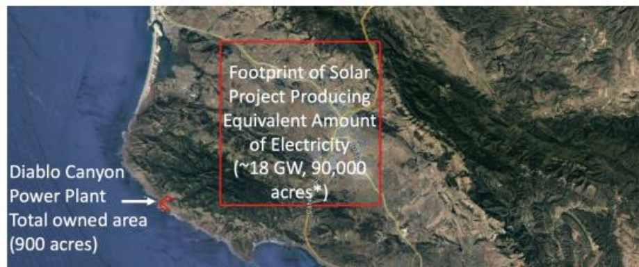
Figure 1.4: Land Area Needed to Produce DCPD Capacity with Solar Energy
