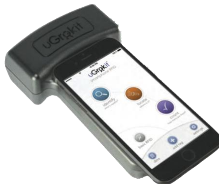
Figure 4: RFID Scanner Attachment for Smart Phone
