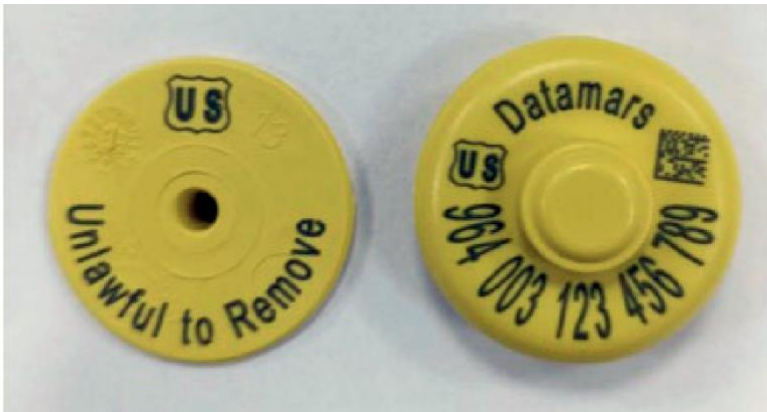
Figure 3: Livestock Ear tag with printed 2D barcode and embedded RFID chip
